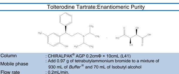
Injection volume : 20μL Column temperature : 25°C UV detection : 220nm *※ Buffer* : Transfer 21.0 mL of 1 M solution of monobasic sodium phosphate and 53.3 mL of 0.5 M solution of dibasic sodium phosphate dehydrate to a 1000 mL volumetric flask, and dilute with water to volume. Dilute 100.0 mL of this solution with water to 1000.0 mL (Buffer solution with pH 7.1)
